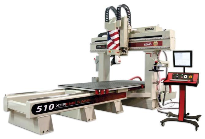
The Xtreme 5 Axis Series of CNC routers from Komo Machine has been developed specifically for the customer who requires more machining flexibility and more Z travel than an Xtreme XL. These machines feature a moving table configuration and 24" of Z travel (standard; 36" optional).
