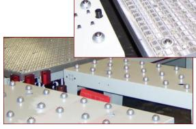
Roller ball table with pneumatic rolling balls for ease of spoil board transfer
