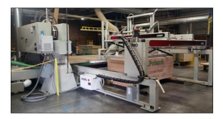
The KOMO Automatic Material Handling System is a fully automatic sheet feeder and unloader designed to be used in nested based manufacturing environments.
