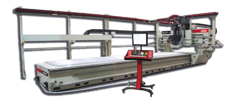
The Mach III GT Series of CNC routers from Komo Machine has been developed specifically for the customer who requires a premier machine with more flexibility, more customizable options and more table than a Mach III. These machines feature a moving gantry with table sizes available up to 120" (3048mm) in the Y axis and 110' (33,000mm) in the X axis, and can be configured with multiple spindles, moulder heads, horizontal spindles etc.
