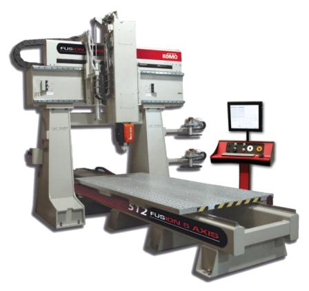
The Fusion 5 Axis Series of CNC routers from Komo Machine has been developed specifically for the customer who requires more machining flexibility and more Z travel than a Fusion XL. These machines feature a moving table configuration and a choice of 36" or 48" Z travel.
