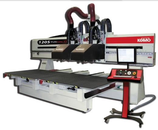
The Fusion Twin Table Series of CNC routers from Komo Machine has been developed specifically for the customer who requires a machine with the flexibility of two tables and one or two spindles. These machines feature a moving table configuration and spindle-mounted tool changers.
