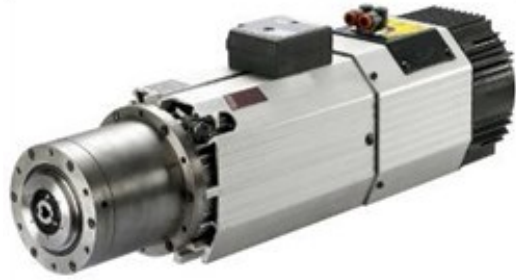
Standard 18HP (13.5KW) S6, 24,000 RPM Fan-Cooled HSD HSK 63F Electro-Spindle
